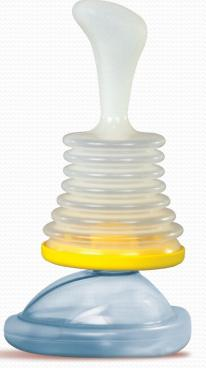
LifeVac is an option if protocol fails. This non-invasive airway clearance apparatus is designed to remove a foreign body obstruction when standard choking protocol has been followed without success. The patented designed valve prevents air from pushing an object or food downward. On the downward compression all air is vented outside the unit. and not into the victim's airway. When the unit is pulled back, negative pressure is generated and it dislodges the obstruction.
